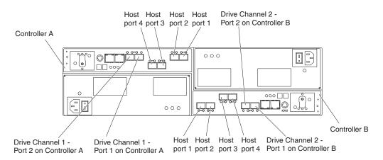
Figure 36. DS5020 storage subsystem ports and controllers
